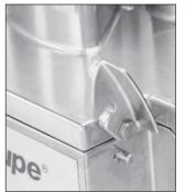
3) Position the head of the vegetable preparation machine on the motor shaft. The fastening hook should now be facing you, on your right.
